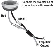
Connect the tweeter as shown in the wiring diagram. Improper connections will cause damage not covered by the product warranty.
